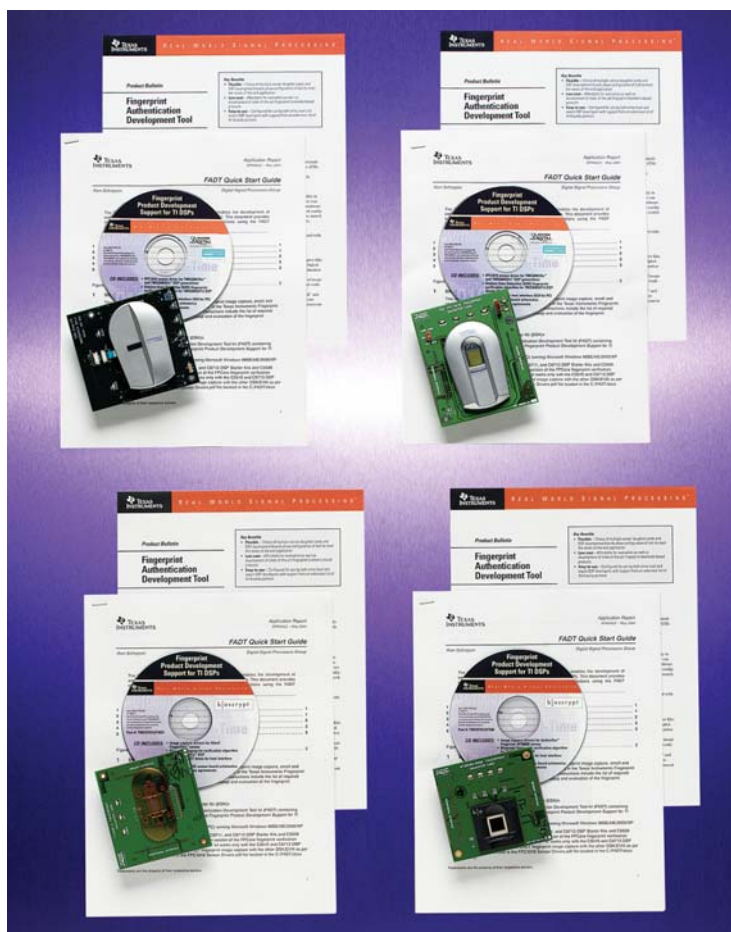
Each FADT includes a sensor daughter card, as well as all the software and documentation to get started. DSP Starter Kits (DSKs) are sold separately.
